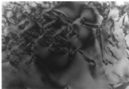
Figure 5. Optical micrograph of the lyotropic solution of polymer 1a (6.3 wt %) in methanesulfonic acid at 25 °C between cross polarizers. The sample was first heated to 120 °C and then cooled slowly to 25 °C.
